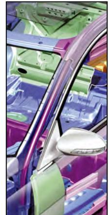
Land Rover LR4, Reinforcement in B-pillar. It's easy to see how you can work around it.
