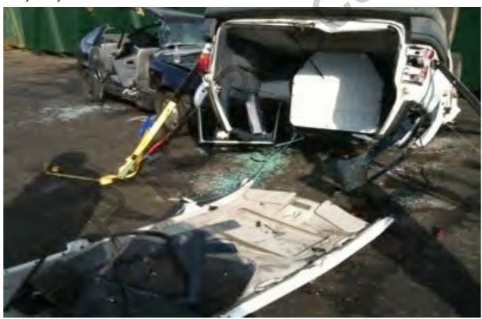
You can see that good vehicle stability will be required to prevent the main chassis from dropping when you make the cuts through the ABCD posts etc
