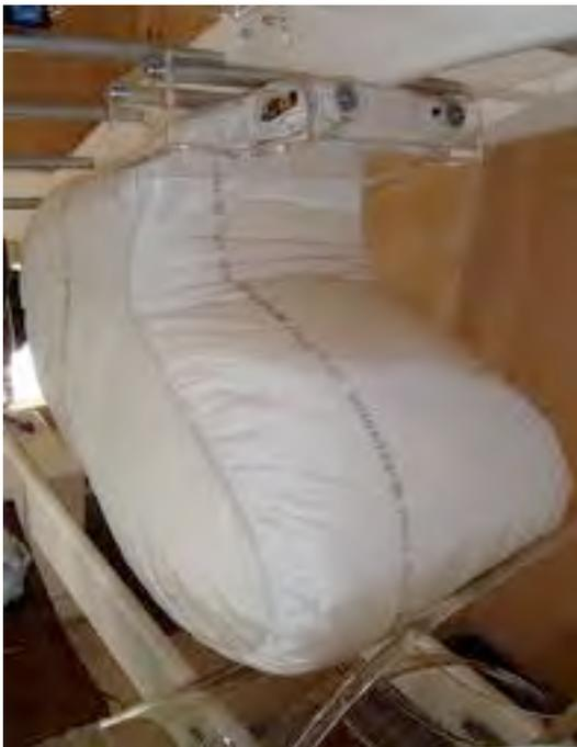
Dubbed the “bag in roof” airbag system, it works by deploying a single airbag large enough to protect both the driver and front seat passenger.
