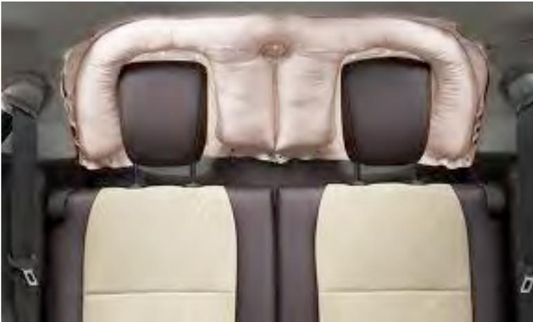
These are found on the Scion IQ as the vehicle is very short and the occupants are very close to the rear window, this airbag works to prevent injury from rear impacts. Normal control measures can be used here, we must as always carry out a thorough scan of the vehicle and expose areas we are working.
