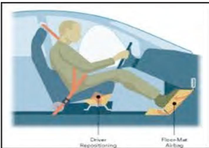
These are designed to prevent submarining of the knees under the dash by lifting the front of the seat. These are either under the seat as seen here or built into the lower seat frame. We need to be aware of these if we are relocating the seat or cutting/ramming in these areas.
