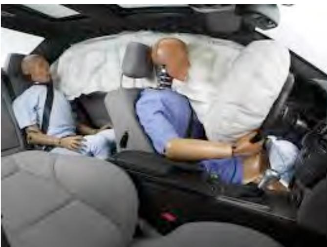
Side airbags will in most cases only deploy from side impacts, however with new vehicles and SMART systems analyzing the crash data it may now be found that these systems may also actuate in a frontal collision, don't forget there may be other forces such as rotational force from rebounds etc.
