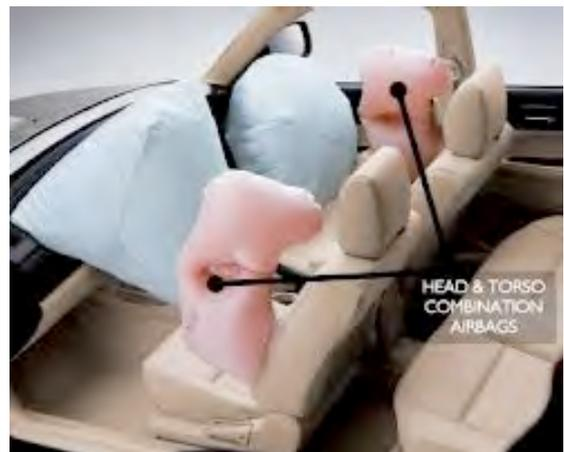
This type of airbag is also a one time activation, once deployed they are safe to work around, these can either be deployed from the B-post, seat or fitted into the door, so a thorough scan for these airbags needs to be carried out.
