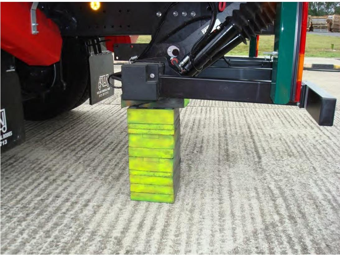
This would be a more suited method covering a greater surface area, and placed onto a load bearing part of the chassis.
