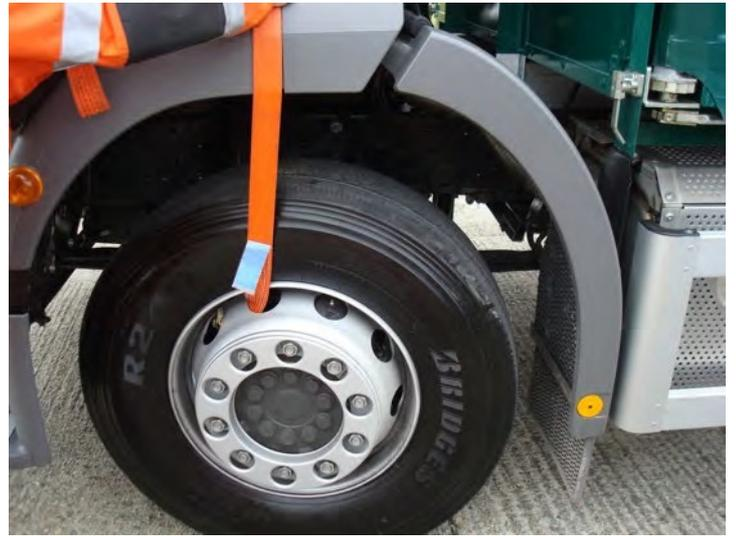
Here we can see the ratchet strap attached to the wheel, either way is ok but you can see that the left hand picture it is attached to the bottom of the wheel, this poses the problem of the wheel turning when tensioned, by law only the rear wheels have to lock when the handbrake is applied, so it would be better to attach the ratchet to the top of the wheel as seen in the right hand picture. Or similarly use a chain set.
