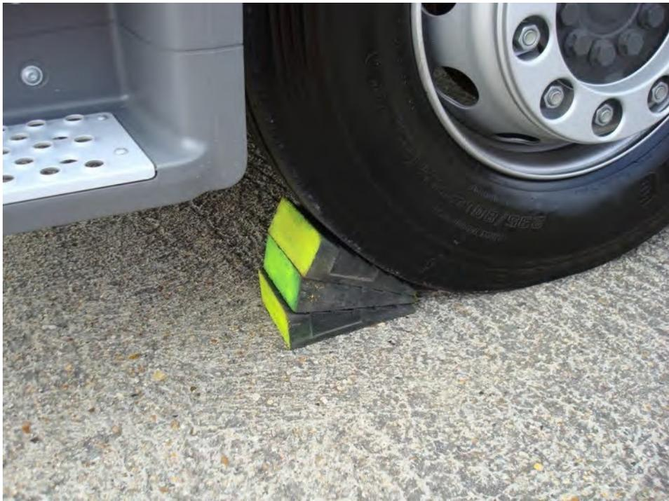
The initial task will be to chock either side of a wheel with suitable wedges big enough to prevent motion.
