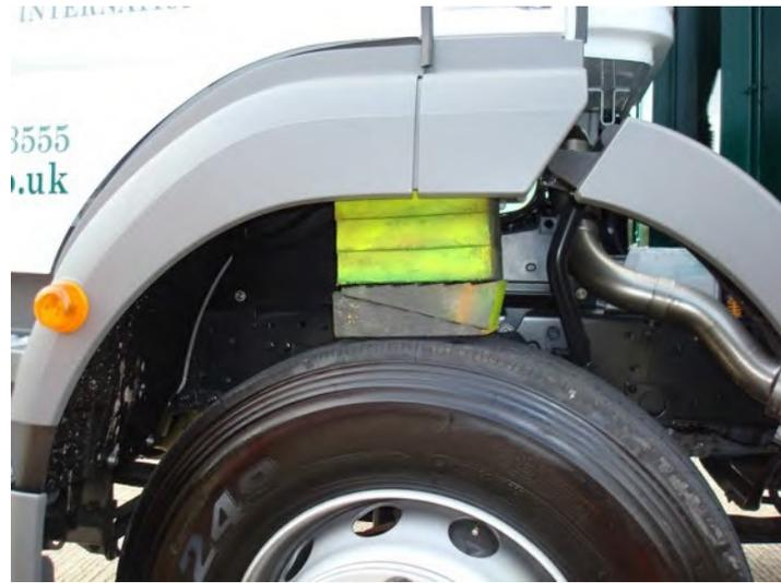
Here you can see the blocks have been placed between the wheel and the top of the wheel arch to provide additional stability for the cab.
