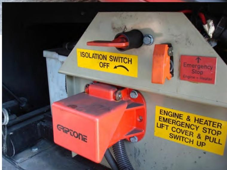
If you still feel that the battery cables need to be disconnected, you can access the batteries from the front or side of the bus. A budget key or screwdriver will normally open the locker where the batteries are kept. Only one set of terminals needs to be disconnected.
