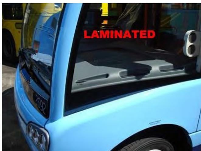
Passenger side windows will be toughened glass and can be dealt with in the same way we do cars, with a center punch and so on.
