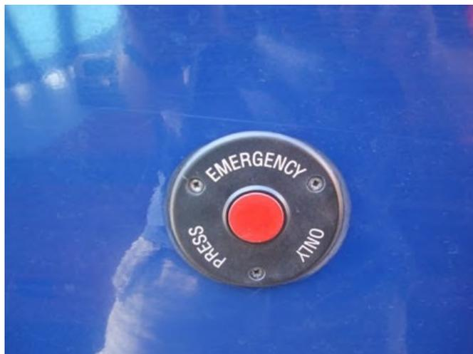
If the system has air in it, you can just push the emergency door release button. However with the door system charged with air there will be a need to secure the door open as it will try and self close.
