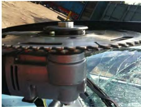
This is the Twin Saw, as you can see it is an electrically powered saw running on either 240v or 110v.
