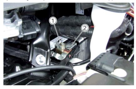
Slacken the nut (1) and pull off the battery earth lead (2) in the upwards direction.
