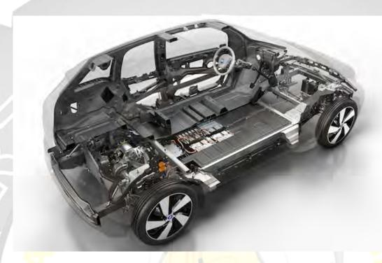
The aluminium chassis will absorb a lot of the crash energy and divert the energy through the structure lessening the stresses that the CFRP may be subjected to.
