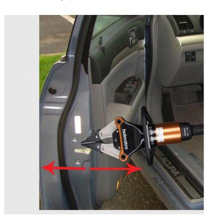
A simple solution that works in most cases is to start above the door hinge at the door cap/ frame and gradually move down so that eventually the spreader tips are spreading the whole of the door outwards and not just some of the skins.
