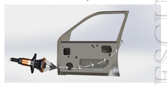
By adjusting the spreading position we can make the door move where we want it to, this is the beauty of extrication, in most cases 'we' facilitate the outcomes.
