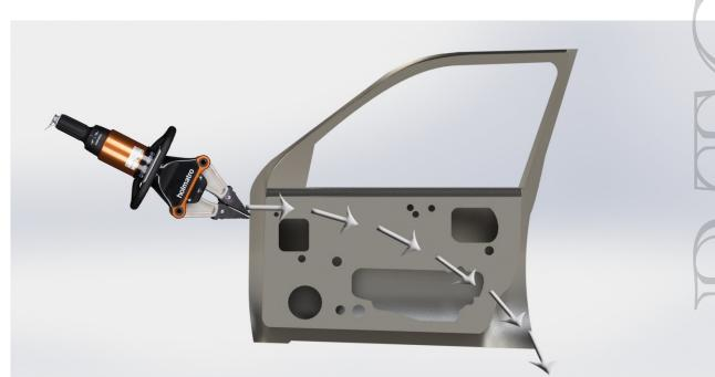
In the same way approaching from the lower hinge can cause the door to move uncontrollably upwards.
