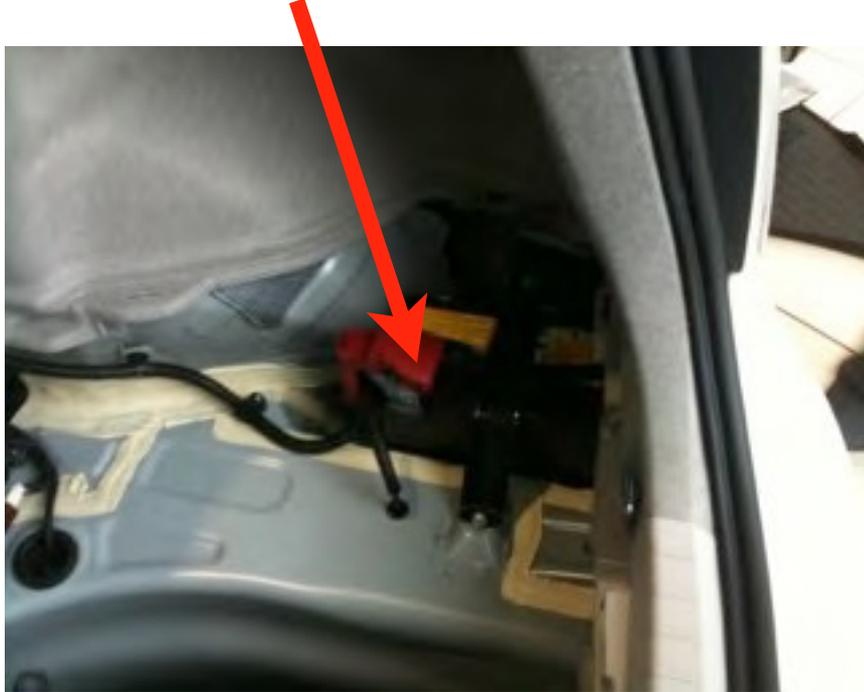
The Orange cables will have a built in safety device so that in the event of a crash they should automatically shut down and self isolate to make them safe, however unless you pull the main plug for the HV battery system they may still be holding 600 volts, so if the safety systems have not activated or we haven't shut down the HV system, they may still be live, if the cables in the engine compartment are touching the bonnet/hood they may energize the whole vehicle, so do not get complacent.
