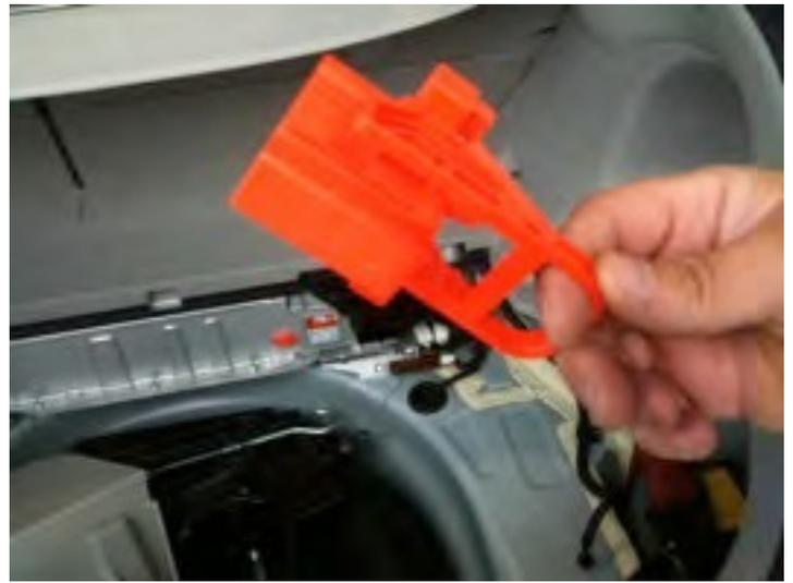
This is the main isolator plug that needs to be removed, you slide it then pull it out, this prevents accidental removal. **It would be a good idea to wear electrical gloves to do this.**
