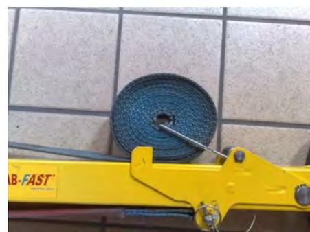
Now you may have found that when you want to extend the main part of the unit it will also require you to pull the strap from the spring holder to give you enough slack to attach the hook to the vehicle, this can be awkward at times as the spring clip can hold the ratchet strap quite firmly.
